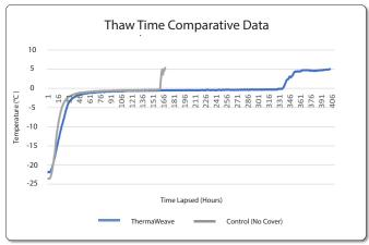
\* Frozen 500lt Pallecon filled with water with Pallet Covers on them, removed from freezer and placed in warehouse.
