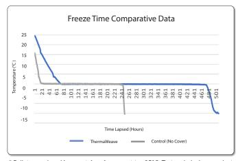
$^{\ast}$  Pallets are placed in a container freezer set to -25°C. Test ended when product reached -15°C.
